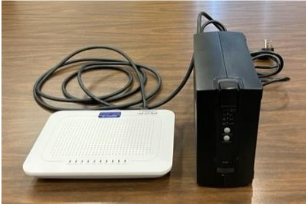
An example fiber ONT (left) and old UPS (right)
